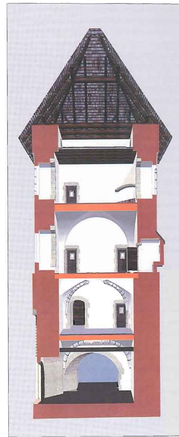
117 Frankopanska kula, presjek sjever-jug, pogled prema istoku, kompjutorska vizualizacija (Studio »Kušan«) Frankopan Tower, north-south section, view to the east, computer visualisation (the Kušan Studio)
