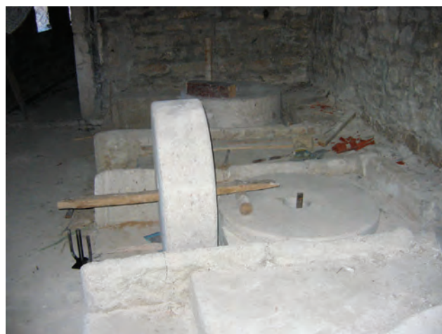
24 Primjena poluge i valjka pri namještanju gornjeg mlinskog kamena (foto: Sanja Buble, 2008.) Application of the rod and cylinder while fitting the upper mill wheel (photo by Sanja Buble, 2008)
