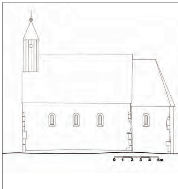
13a i 13b Hipotetička rekonstrukcija crkve, tlocrt i južno pročelje. Analiza autora prema nalazima konzervatorskih istraživanja (crtao Damir Zahirović) 13a and 13b Hypothetical reconstruction of the church, ground-plan and south elevation. Author's analysis according to the findings of conservation research (drawn Damir Zahirović)
